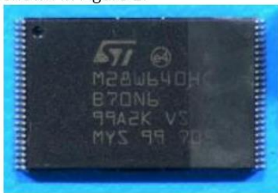
Figure 1. Authentic IC component that has undergone the standard Dynasolve 750 test at Global Electronic Testing Services-USA. The left section represents the package before testing and the right section represents the package after testing. The original manufactured package has been damaged and this is one example of hundreds.
